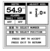
instead of the surface. To do this, measure the lowest part of the boat below the transducer. In this example, we'll use 3 feet. Now, using the keel offset feature, adjust the offset for a *negative* 3 feet.
